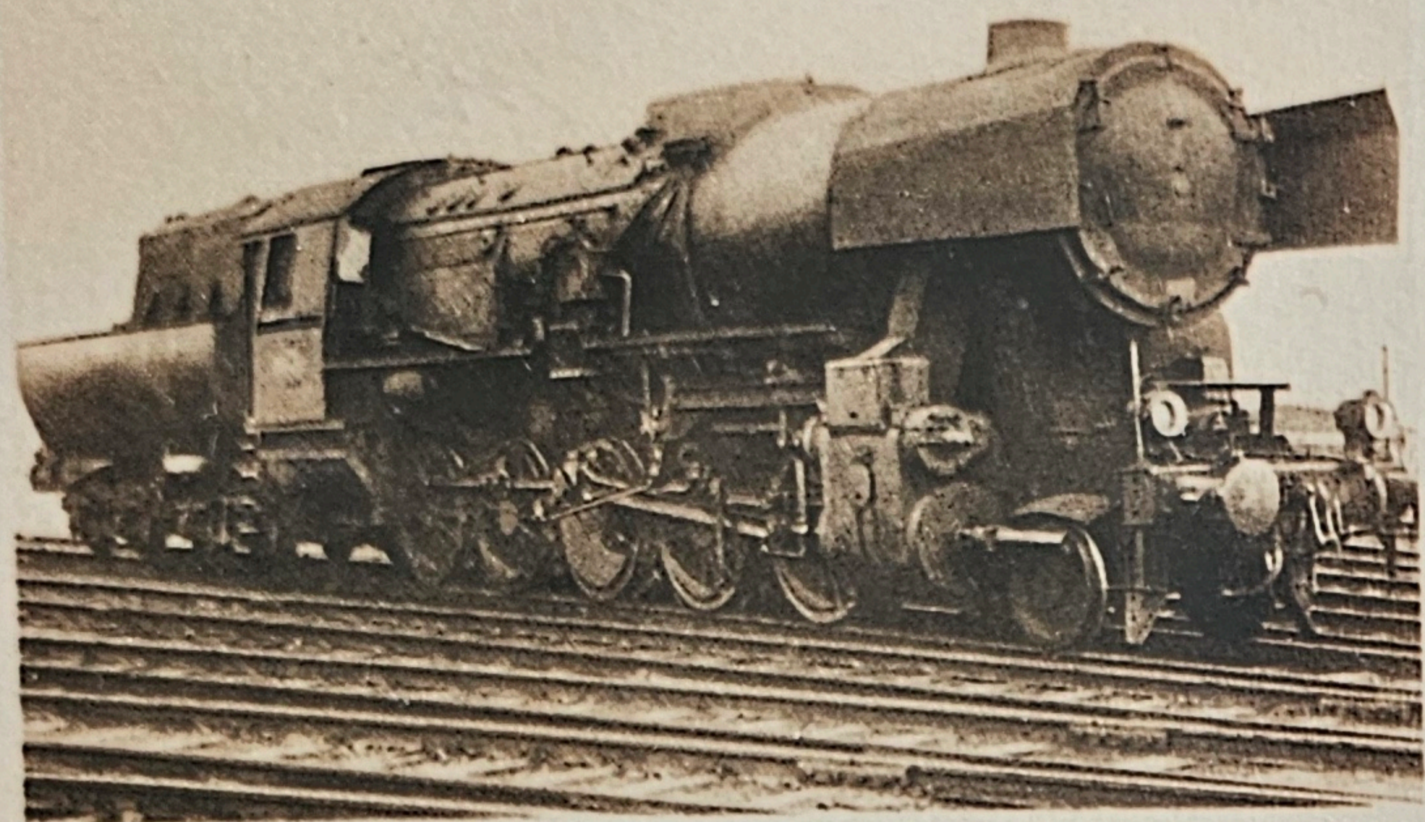
LOCOMOTIVE Type 150 Y "DECAPOD" Tender 32 Y - 2 cylindres HP
