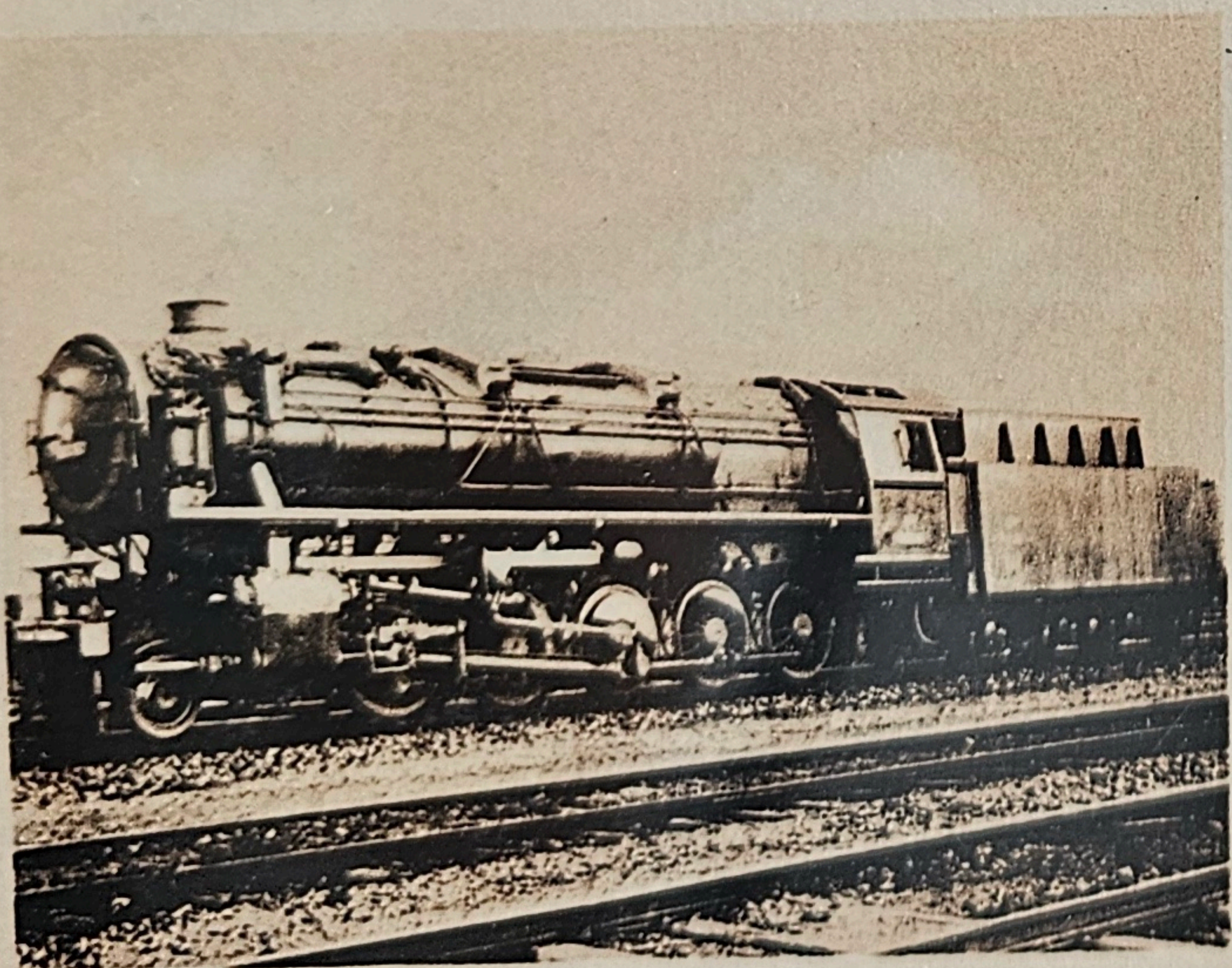
LOCOMOTIVE Type 150 X "DECAPOD" Tender 34 X à 3 cylindres HP
